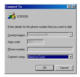
Next you have to choose the communication settings of the Com port. The settings are 115,2 kBaud, 8 databits, 1 stopbit, no parity, protocol none. You should see a window similar like this:
